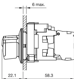
Selector switch long lever (flush design)
