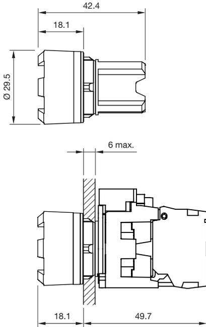
Double pushbutton, Lens level with front ring (raised design)
