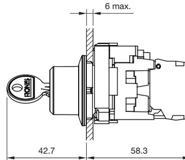
Selector switch short lever (flush design)
