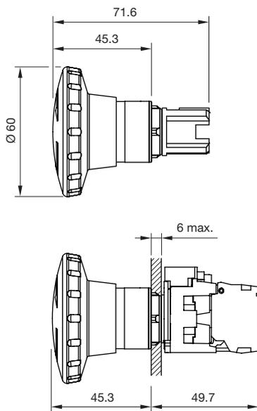
Emergency stop switch with key  $\varnothing$  40 mm
