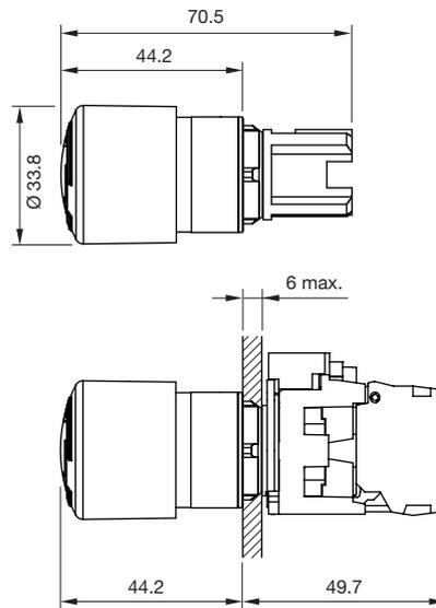
Emergency stop switch, Stop switch  $\varnothing$  40 mm
