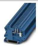
Feed-through terminal block, Connection type: Screw connection, Cross section: 0.14 mm² - 6 mm², AWG: 26 - 10, Nominal current: 20 A, Nominal voltage: 500 V, Length: 57.8 mm, Width: 6.2 mm, Color: blue, Assembly: NS 35/7,5, NS 35/15
