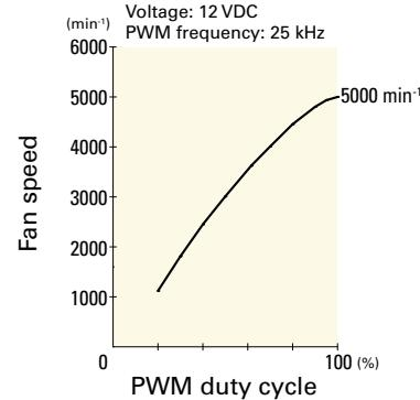
**9GA0824P7G001** With pulse sensor with PWM control function
