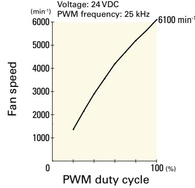
**9GA0824P7S001** With pulse sensor with PWM control function
