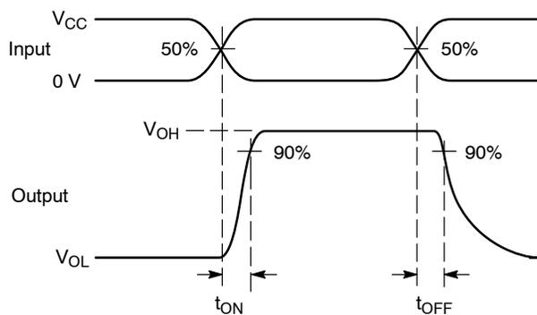
Figure 3.  $t_{ON}/t_{OFF}$
