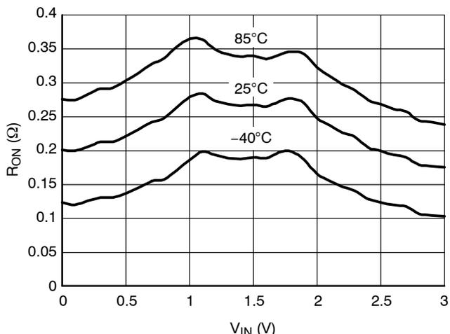
Figure 10. On-Resistance vs. Input Voltage
