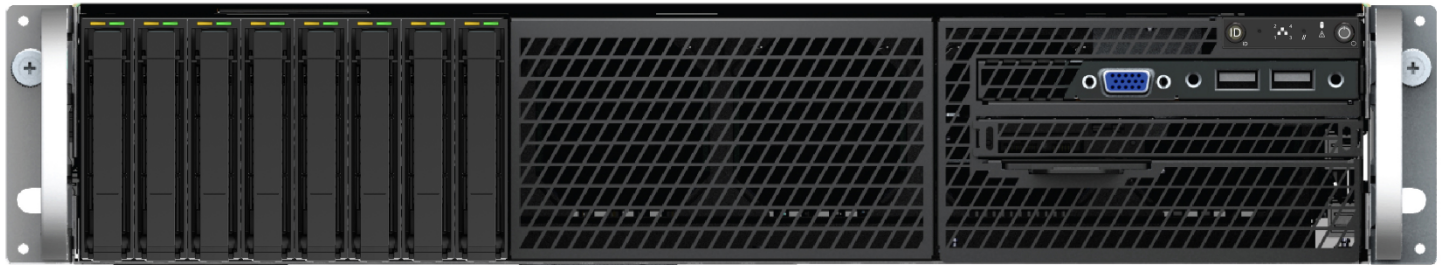
Figure 12. 2.5" x 8 front drive bay configuration – R2208WFxxxx
