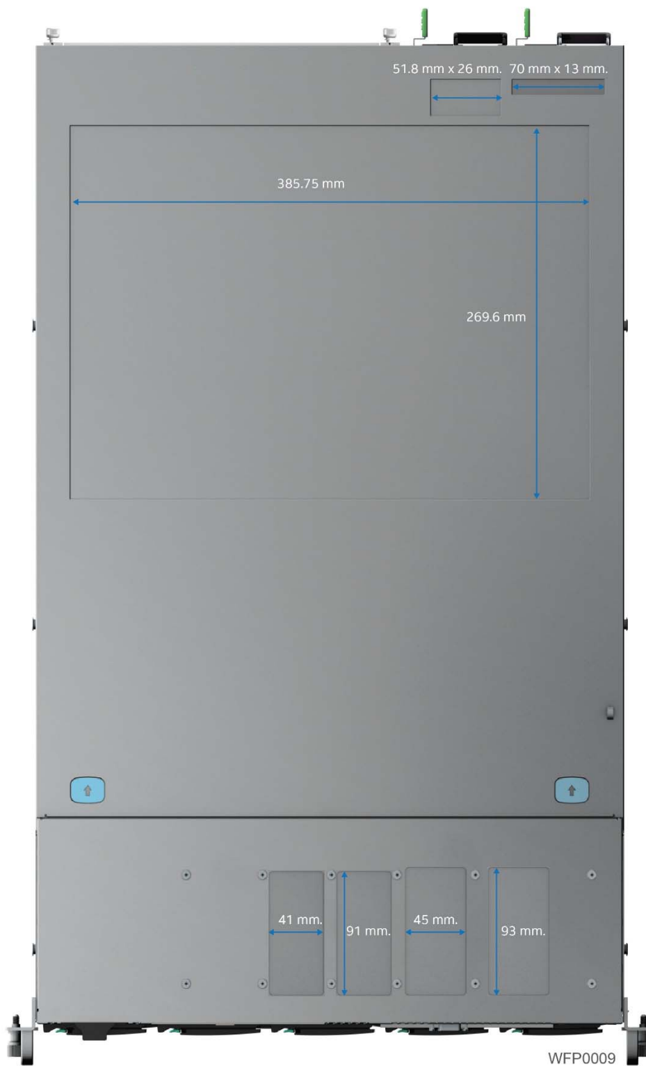
Figure 17. Label emboss dimensions
