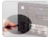
Plug ring-lock securely fastens the power cord
