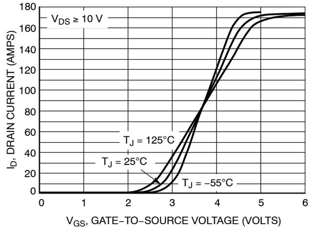
Figure 2. Transfer Characteristics
