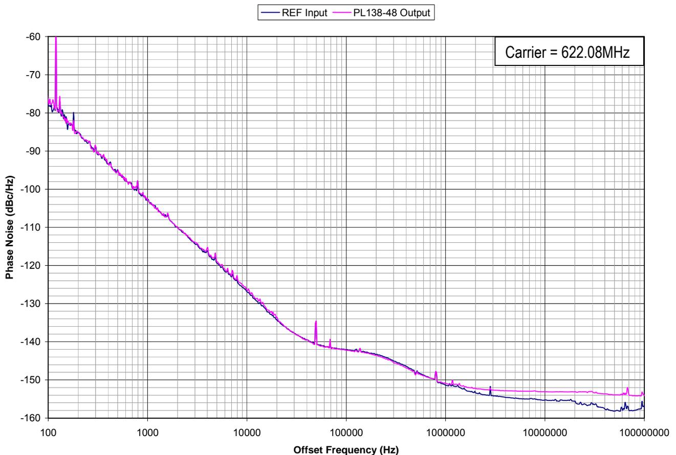
When a buffer is used to pass a signal then the buffer will add a little bit of its own noise. The phase noise on the output of the buffer will be a little bit more than the phase noise in the input signal. To quantify the noise addition in the buffer we compare the Phase Jitter numbers from the input and the output. The difference is called "Additive Phase Jitter". The formula for the Additive Phase Jitter is as follows:
