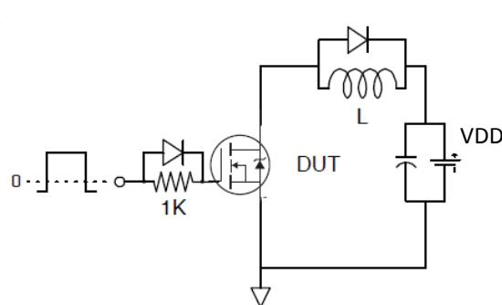
**Fig 25a.** Gate Charge Test Circuit
