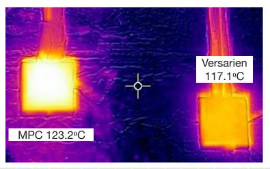
Comparative heatmap of a 40x40x2.5 microporous ceramic and VersarienCu<sup>TM</sup> heat sink at 5W. The Versarien heat sink is  $6.1^{\circ}$ C/W cooler.
