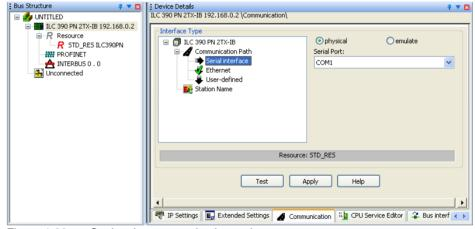
Figure 4-30 Setting the communication path
