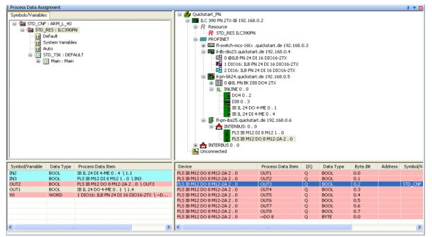
Figure 6-7 All used process data assigned to variables
