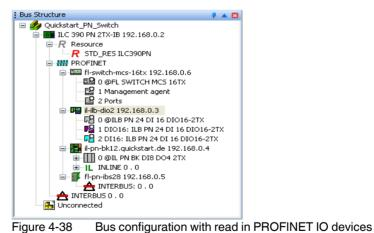
The PROFINET structure is displayed in the "Bus Structure" window.
