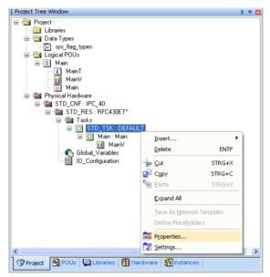
Figure 7-9 Standard task: Properties
