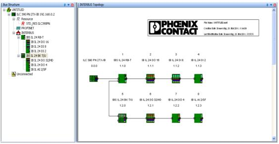
PC WorX can be used to automatically detect INTERBUS topologies. The INTERBUS structure can be viewed in the "INTERBUS Topology" window.
