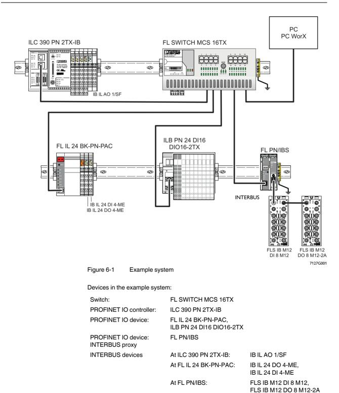
Several PROFINET IO controllers can be used within a project. In this example, only one PROFINET IO controller is used.
