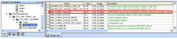
Figure B-5 PNIO\_FORCE\_FAILSAFE system variable
