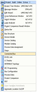
Figure 4-43 "View, Connected Bus" command
