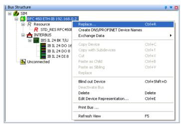
Figure A-3 Replacing a device
