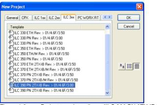
Figure 4-2 Project templates (here: "ILC 390 PN 2TX-IB Rev. > 01/4.6F/3.00")
