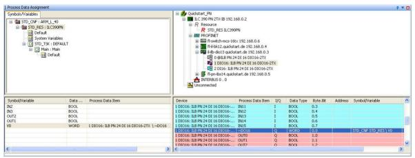
Figure 4-23 Assigning process data for a PROFINET IO device
