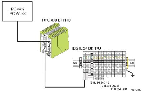
Figure 7-1 Example bus configuration
