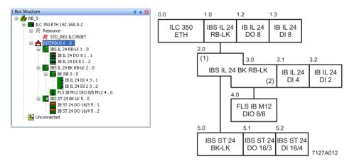
Example 3: Bus configuration with bus coupler for connecting a remote bus branch
