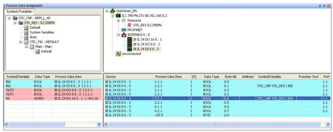
Figure 5-4 All used process data assigned to variables
