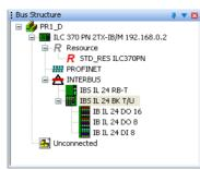
Figure A-7 Bus configuration with new controller
