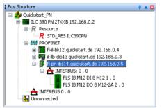
Figure 4-16 FLM modules inserted below an INTERBUS proxy
