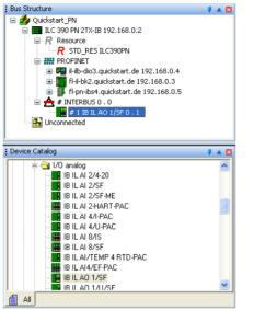
Figure 4-12 Device inserted (here: IB IL AO 1/SF)
