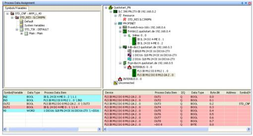
Figure 4-24 All used process data assigned to variables
