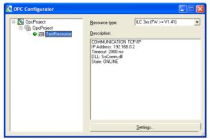
Figure C-8 OPC configuration completed
