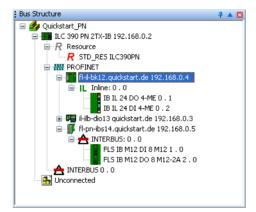
Figure 4-17 Inline terminals inserted below a PROFINET IO bus coupler
