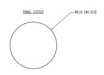
\*UNLESS OTHERWISE SPECIFIED TOLERANCES PER DECIMAL PRECISION ARE: X=±1 (±0.039), X.X=±0.5 (±0.020), X.XX=±0.25 (±0.010), X.XXX=±0.127 (±0.005). LEAD SIZE=±0.05 (±0.002), LEAD LENGTH=±0.75 (±0.030). MIN=  $^{+0.00}_{-0.00}$  PRECISION MAX.=  $^{+0.00}_{-0.00}$  MAX.=  $^{+0.00}_{-0.00}$  PRECISION ARE: X=±1 (±0.039), X.XX=±0.5 (±0.001), X.XXX=±0.127 (±0.005). LEAD SIZE=±0.05 (±0.002), LEAD LENGTH=±0.75 (±0.030). MIN=  $^{+0.00}_{-0.00}$  PRECISION MAX.=  $^{+0.00}_{-0.00}$  PR
