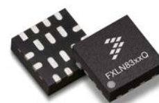
12-pin QFN 3 mm x 3 mm x 1 mm Case 2300-01
