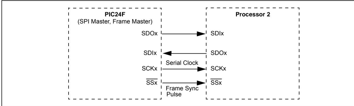
**FIGURE 16-6: SPI MASTER, FRAME SLAVE CONNECTION DIAGRAM**
