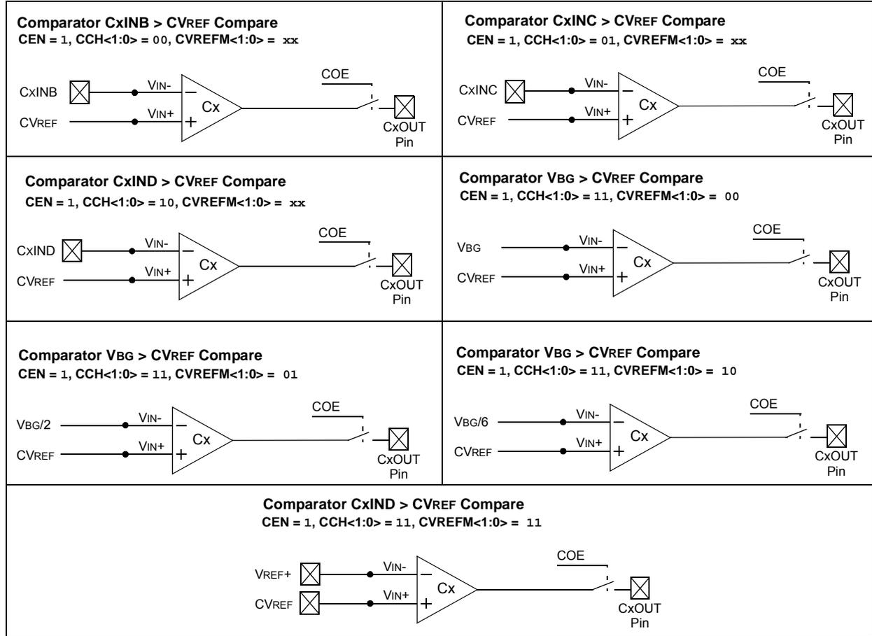
**FIGURE 25-4: INDIVIDUAL COMPARATOR CONFIGURATIONS WHEN CREF = 1 AND CVREFP = 1**
