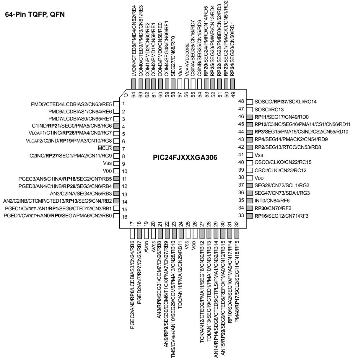
**Legend:** RPn and RPin represent remappable pins for Peripheral Pin Select feature. Shaded pins indicate pins that are tolerant up to +5.5V.
