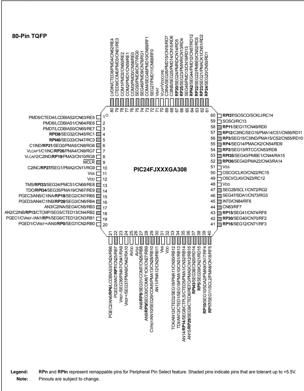
**Legend:** RPn and RPI n represent remappable pins for Peripheral Pin Select feature. Shaded pins indicate pins that are tolerant up to +5.5V.
