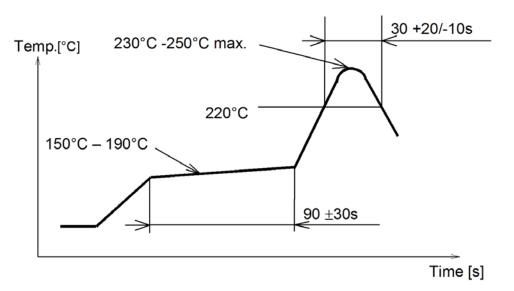
Reflow permissible cycle: 2 Opposite side reflow is prohibited due to module weight.
