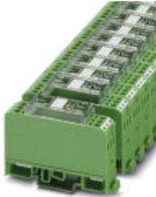
Relay module, with soldered-in remanence miniature switching relay, with positive switching diode wiring, contacts (AgSnO): small to large loads, 1 PDT, 60 V DC input voltage
