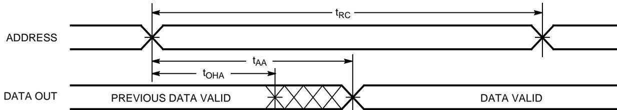
Figure 5. Read Cycle 2 ( $\overline{\text{OE}}$  Controlled) [22, 23]
