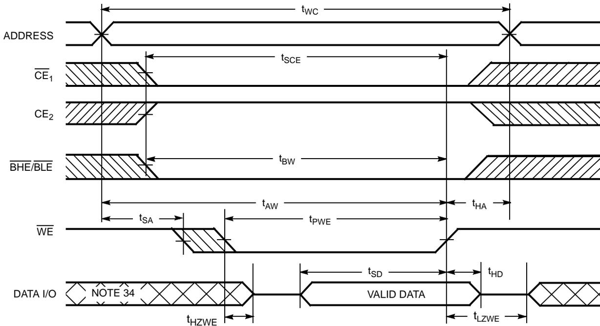
Figure 9. Write Cycle 4 ( $\overline{BHE}/\overline{BLE}$  Controlled,  $\overline{OE}$  LOW) [32]
