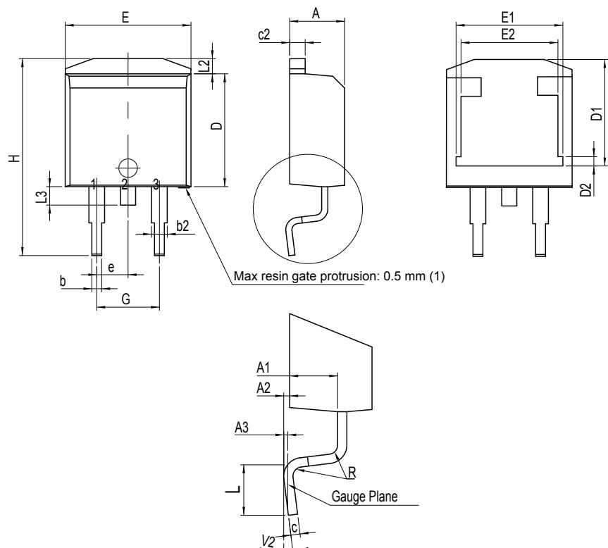
(1) Resin gate is accepted in each of position shown on the drawing, or their symmetrical.
