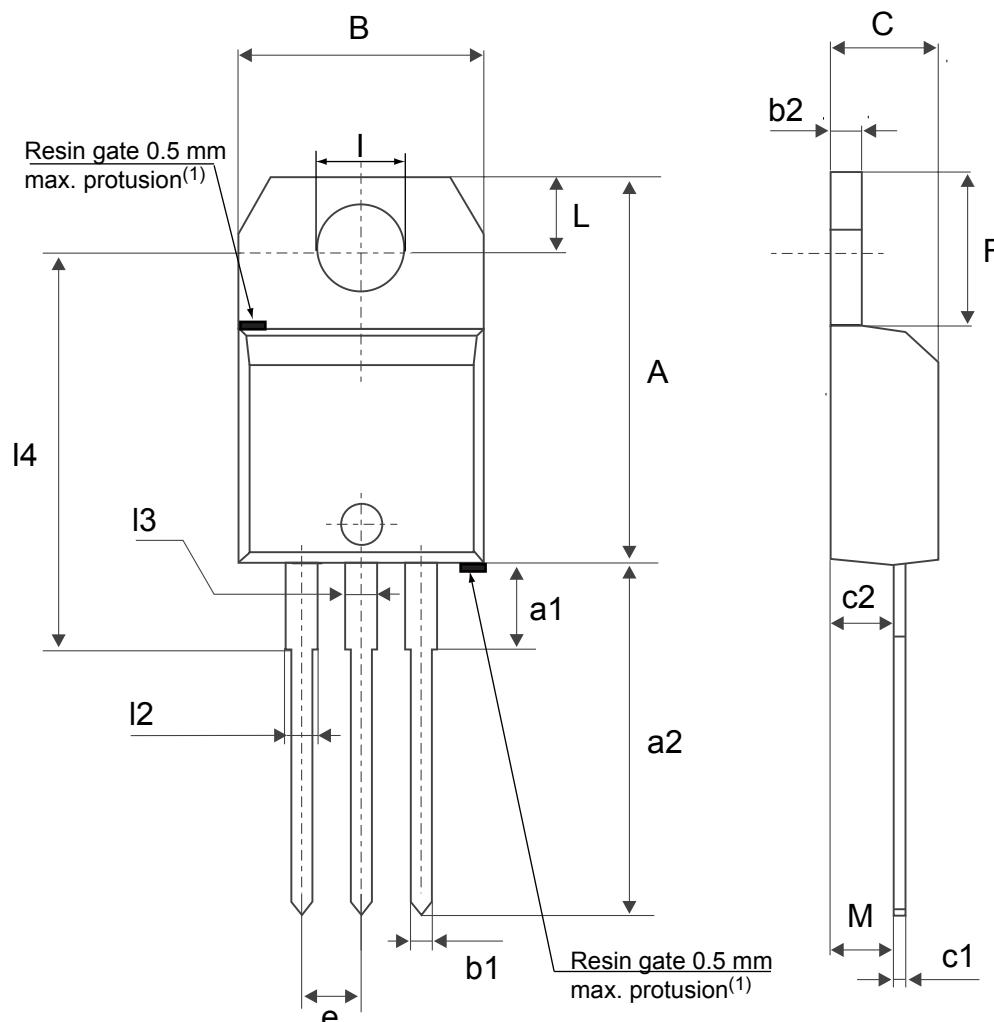
(1)Resin gate position accepted in one of the two positions or in the symmetrical opposites.
