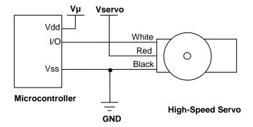
$V\mu$  = microcontroller voltage supply
