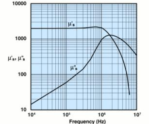
Measured on an 18/10/6mm toroid using the HP 4284A and the HP 4291A.
