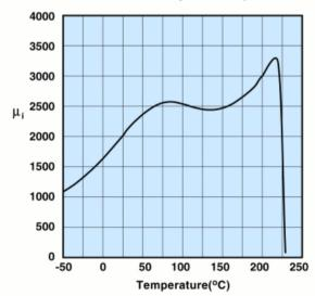
Measured on an 18/10/6mm toroid at 100kHz.
