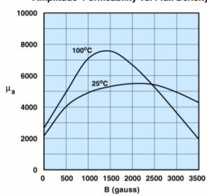
Measured on an 18/10/6mm toroid at 10kHz.
