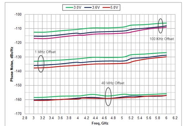
**Figure 7. Single sideband integrated phase noise vs. frequency and supply ( $F_{PFD} = 50$  MHz)**
