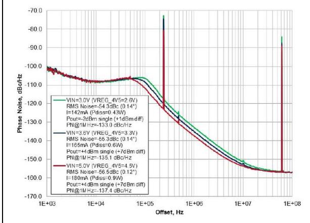
**Figure 10. Phase noise and fractional spurs at 2118.24 MHz vs. supply ( $F_{PFD} = 61.44$  MHz)**
