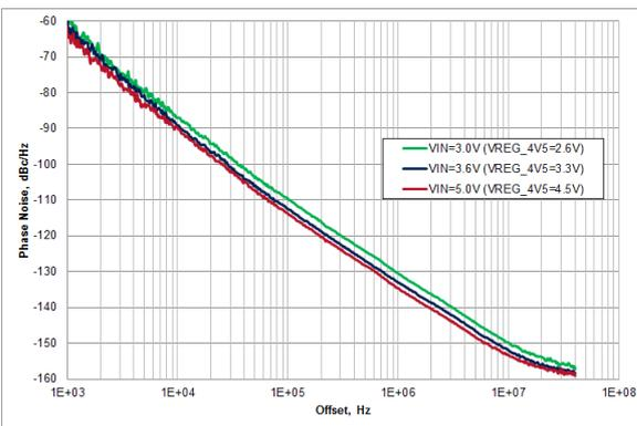
**Figure 6. VCO open-loop phase noise over frequency vs. supply**
