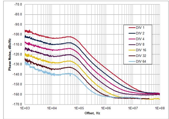
**Figure 5. VCO open-loop phase noise at 4.4 GHz vs. supply**
