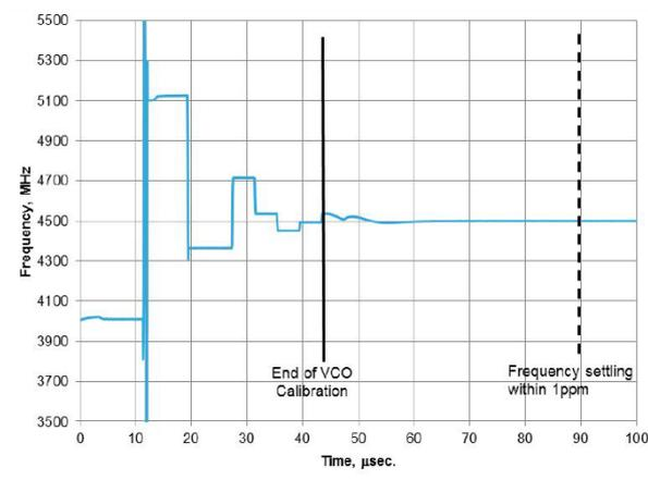
Figure 24. Frequency settling with VCO calibration – narrowband view
