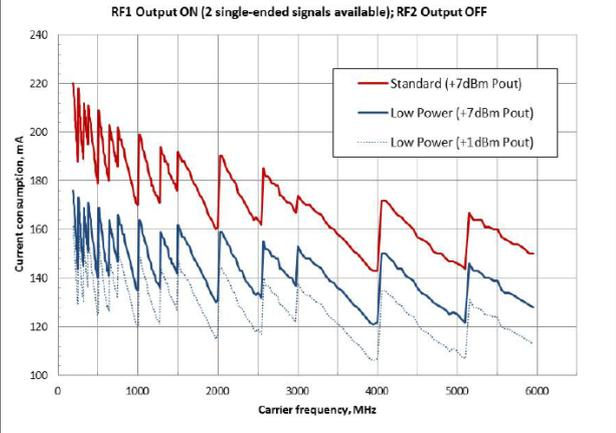
**Figure 27. Current consumption – standard vs. low power (3.6 V supply,  $F_{PFD} = 50$  MHz)**
