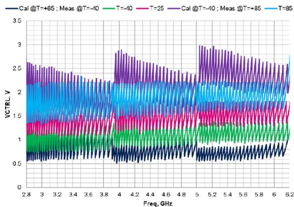
**Figure 16. Average  $K_{VCO}$  over VCO frequency and supply**
