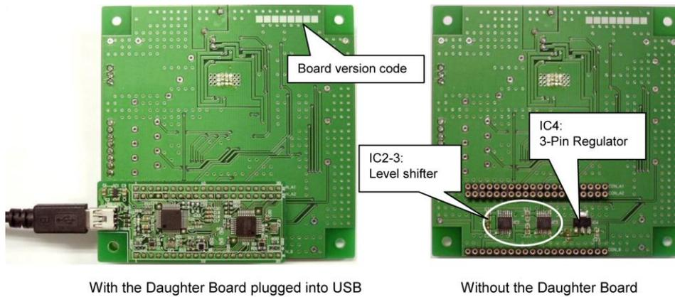
Figure 2. Bottom view of the Evaluation Board
