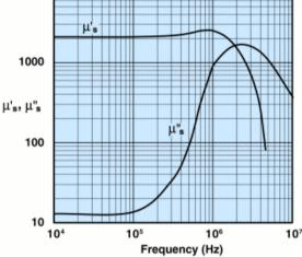
Measured on an 18/10/6mm toroid using the HP 4284A and the HP 4291A.
