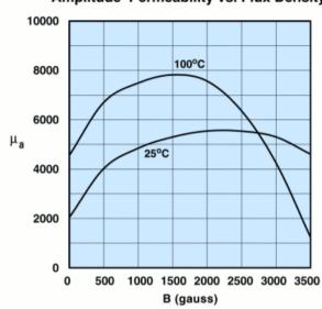
Measured on an 18/10/6mm toroid at 10kHz.
