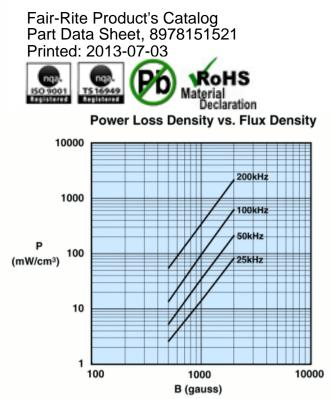
Measured on an 18/10/6mm toroid using the Clarke Hess 258 VAW at 100°C
