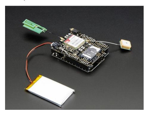
This shield fits right over your Arduino or compatible. At the heart is a powerful GSM cellular module (we use the latest SIM808) with integrated GPS. This module can do just about everything
