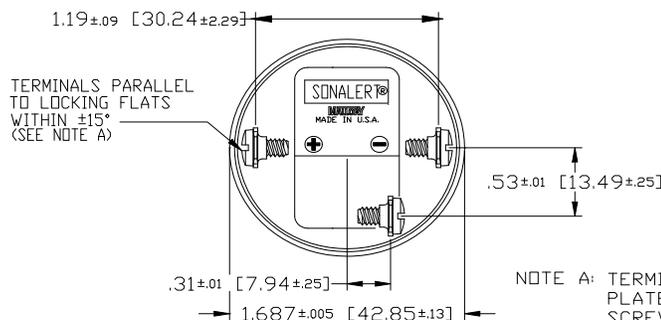
NOTE A: TERMINALS-.032 BRASS TIN PLATED, TAPPED FOR #6-32 SCREW. TWO #6-32 NICKEL PLATED BRASS SCREWS INCLUDED. WILL ACCEPT 1/4" QUICK CONNECT.
