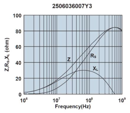
Impedance, reactance, and resistance vs. frequency.
