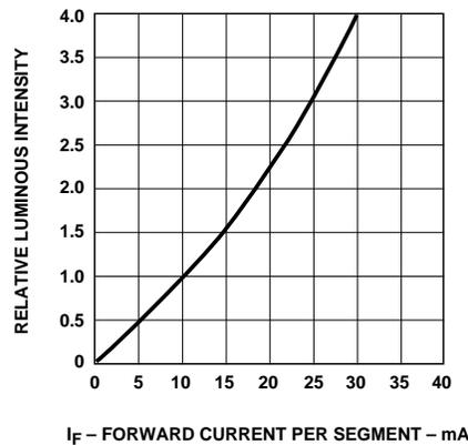
Figure 12. Relative Luminous Intensity vs. DC Forward Current.
