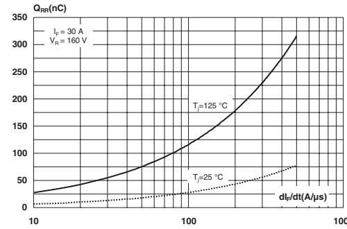
**Figure 8. Peak reverse recovery current versus  $\text{d}I_F/\text{dt}$  (typical values)**
