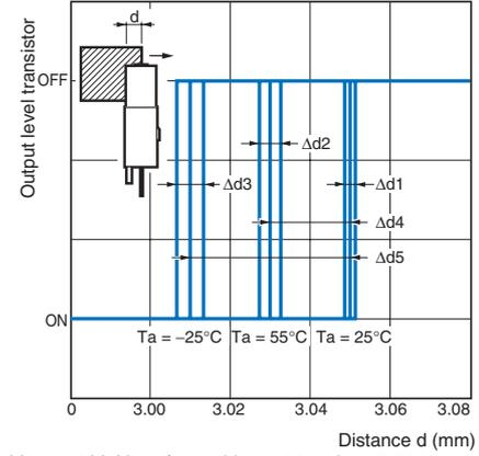
Vcc = 12 V, No. of repetitions: 20, Δd1 = 0.002 mm, Δd2 = 0.004 mm, Δd3 = 0.005 mm, Δd4 = 0.02 mm, Δd5 = 0.04 mm
