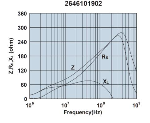
Impedance, reactance, and resistance vs. frequency.
