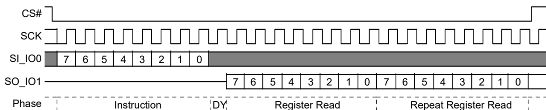
Figure 53. DLP Read (DLPRD) Command Sequence
