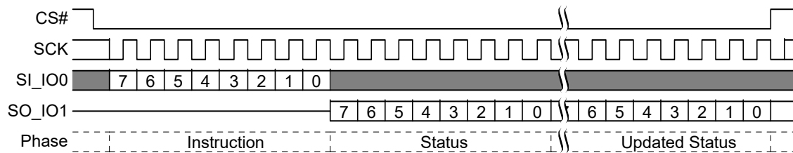
Figure 35. Read Status Register 1 (RDSR1) Command Sequence
